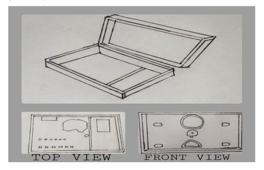
Figure 1 Shows the Design of Improvised Motorcycle Electrical Trainer
