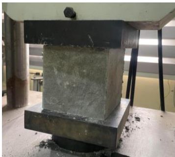
Figure 1 Compressive Strength Testing using a Universal Testing Machine.
